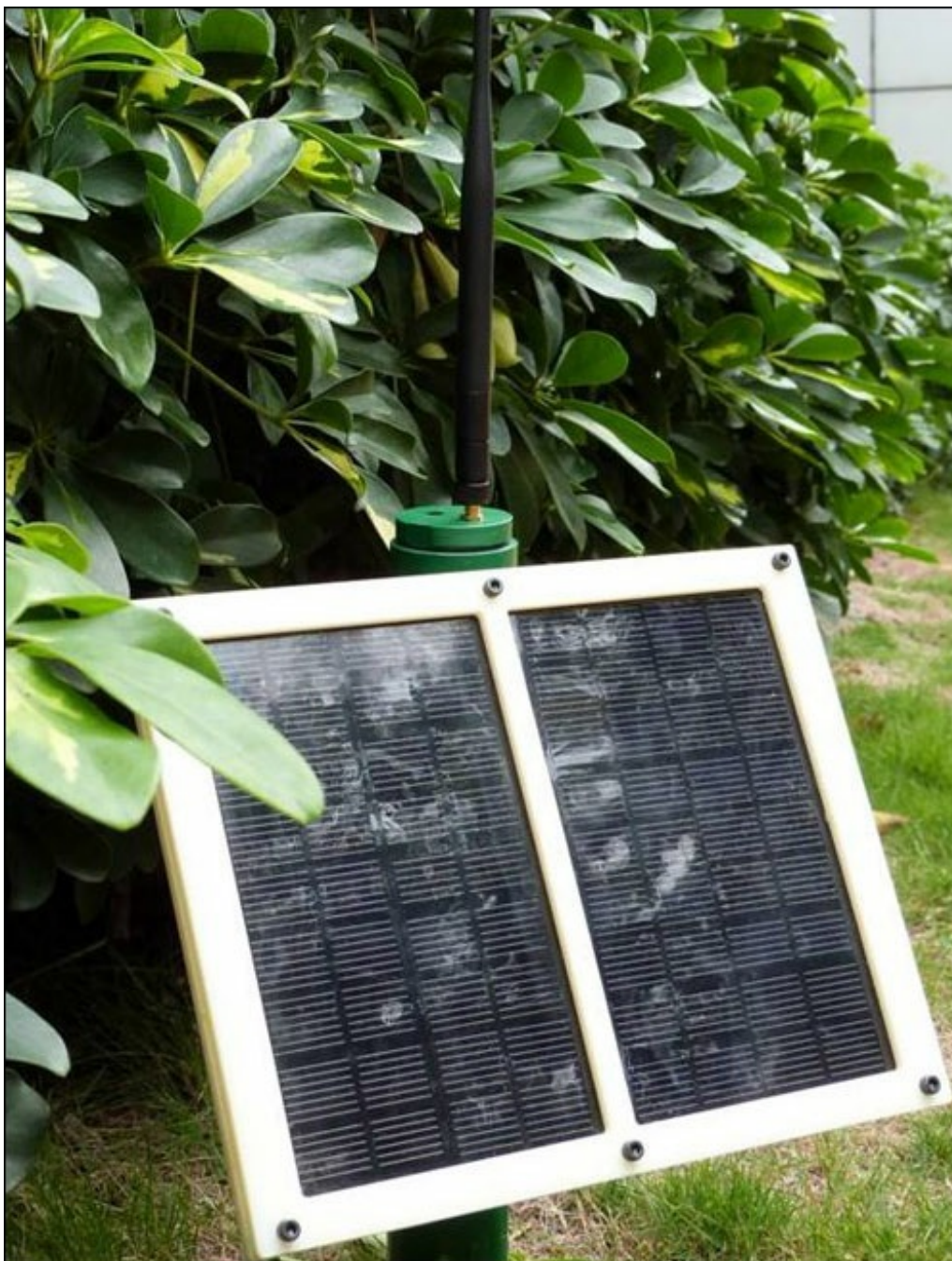
An Insight Robotics wireless sensor and solar panel mounted on a pole
