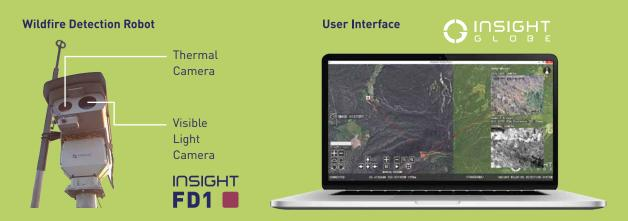
Our proprietary wildfire detection algorithm dynamically adjusts the thermal sensor's threshold to minimise false alarms and increase accuracy. Armed with geographic information and smart algorithms, our robots are able to make sophisticated detection decisions, in low visibilities and without human assistance.
